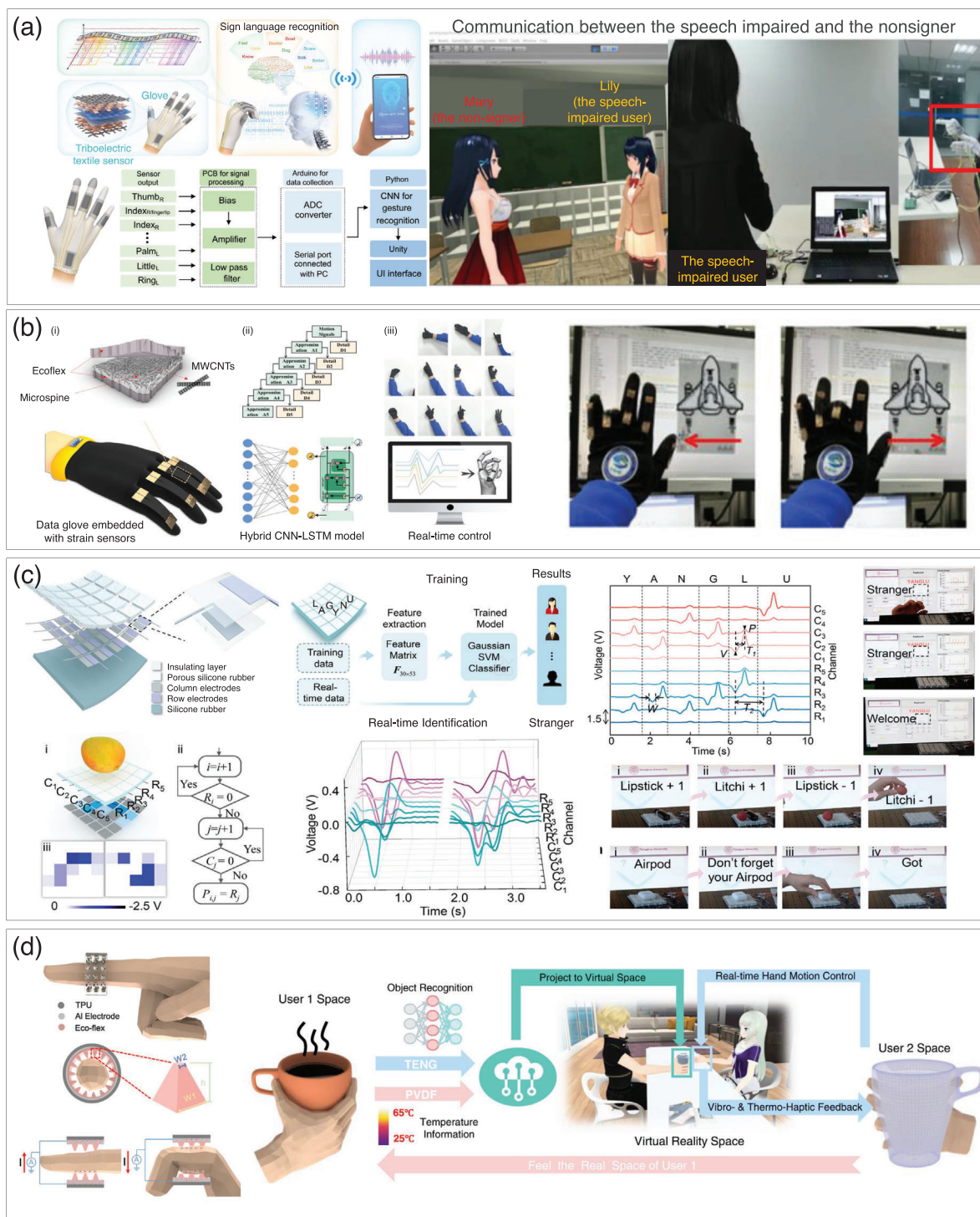
Figure 9. ML-enhanced Sensors for human motion monitoring. a) A triboelectric smart glove integrated with ML algorithms capable of reconstructing unseen sentences, enabling sign language translation and facilitating real-time communication in virtual reality environments, reproduced under the terms of the CC-BY-4.0 license, [129] Copyright 2021, The Author(s). b) A low-cost data glove employing a deep-learning hybrid CNN-LSTM model for gesture-based controls in smart vehicles, improving robotic dexterity, and supporting immersive interactions in virtual and augmented reality systems, reproduced under the terms of the CC-BY-4.0 license, [134] Copyright 2022 The Authors. Advanced Intelligent Systems, published by Wiley-VCH GmbH. c) Bioinspired triboelectric soft sensor arrays utilizing MLP for applications in industrial automation, smart home management, and rehabilitation monitoring, reproduced under the terms of the CC-BY-4.0 license, [135] Copyright 2022, American Chemical Society. d) Augmented Tactile-Perception Ring incorporating triboelectric and pyroelectric sensors for gesture recognition and temperature sensing, designed for use in metaverse applications, robotic systems, and rehabilitation therapies, reproduced under the terms of the CC-BY-4.0 license, [137] Copyright 2022, The Author(s).
